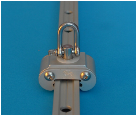
No. 02341 Car body in aluminium (6082 T6) Anodised minimum 25 my in natural/silver colour End caps in aluminium 5 mm shackle
