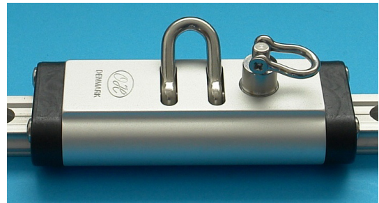
No. 02248/03048 Car body in aluminium (6082 T6) Anodised minimum 25 my in natural/silver colour End caps in delrin Adjustable stop in stainless steel (AISI 316)
