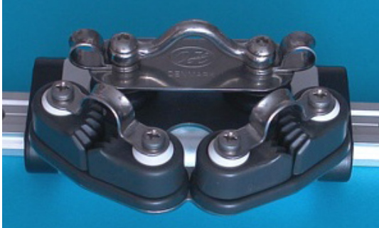
No. 02292 Car body in aluminium (6082 T6) Anodised minimum 25 my in natural/silver colour End caps in delrin
